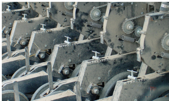
Figure 5. Seed metering for seed singulation on a grain drill. Meter device is shown with gear and chain drive (see fig. 6 for location).
