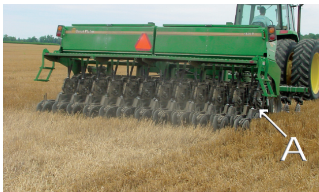
Figure 6. Precision seeding system with seed meters close to the ground ("A" marks the metering device).
