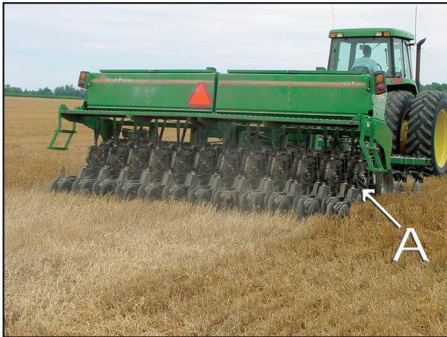
Figure 6. Precision seeding system with seed meters close to the ground. ("A" marks the metering device).
