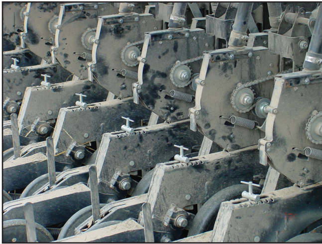
Figure 5. Seed metering for seed singulation on a grain drill. Meter device is shown with gear and chain drive (see Figure 6 for location).
