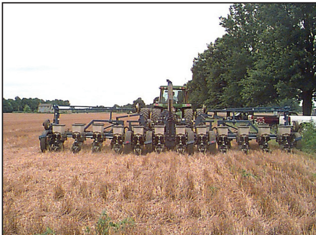
Figure 7. Planter equipped with extra planter boxes to plant 15-inch rows.
