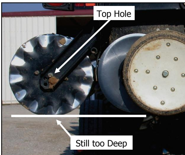
**Closing Wheel Arm Settings.** Once the seed has been positioned at a consistent depth to promote uniform emergence, it is critical to close both sides of the seed slot to optimize seed to soil contact and promote even emergence.
