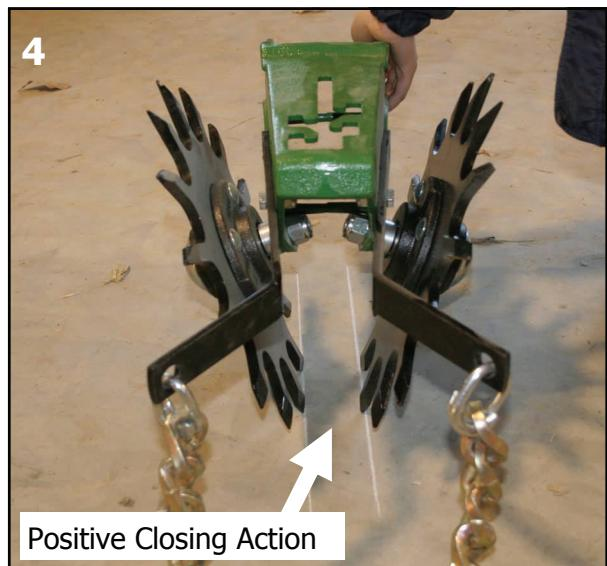
The closing wheel arm angle is very important for the closing action of planters, especially when trying to close the seed slot in difficult conditions. As the rear of the closing wheel arm lowers, the gathering action of the closing wheels is reduced, in fact at a point around 10 degrees less than horizontal, it changes to a negative gathering action which makes closing the seed slot almost impossible in difficult conditions.
